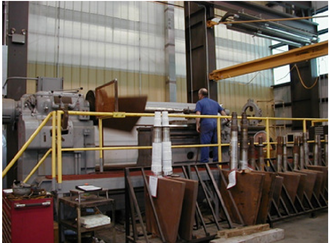
Overhaul of 110 Rudders and Fins for U.S.C.G. in "gap" lathe
